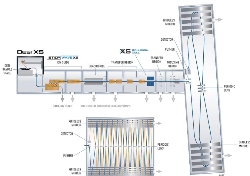
Figure 1: SELECT SERIES MRT instrument schematic.
