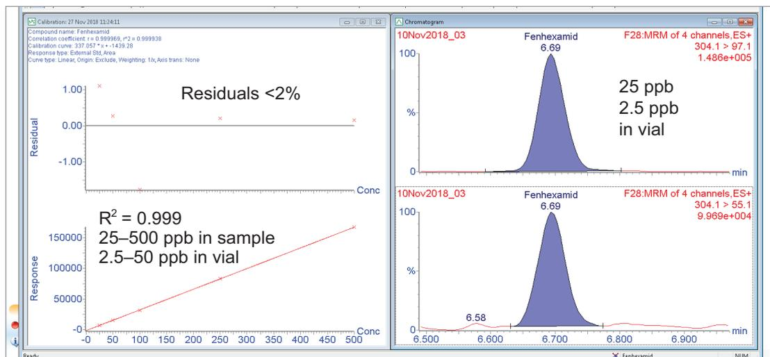
Figure 3. Representative example of a quantitation curve for fenhexamid, demonstrating a linear range from 0.025 to 0.50  $\mu\text{g/g}$  (25 to 500 ppb in sample or 2.5 to 50 ppb in vial concentration).
