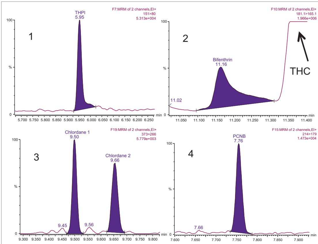
Figure 7. Representative MRM chromatograms for (1) THPI, captan degradation product; (2) bifenthrin; (3) trans and cis chlordane; (4) PCNB spiked at a level of 0.1 µg/g in cannabis flower (0.7 µg/g for THPI) and extracted using the sample preparation protocol reported.
