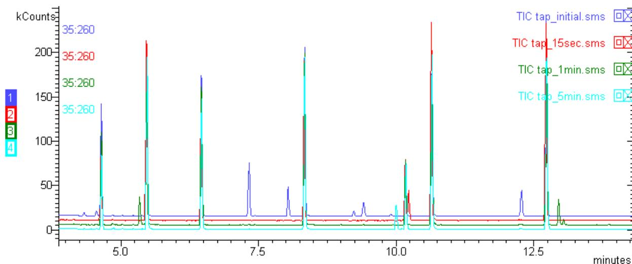
Figure 2: Tap Water VOC Comparison over Time
