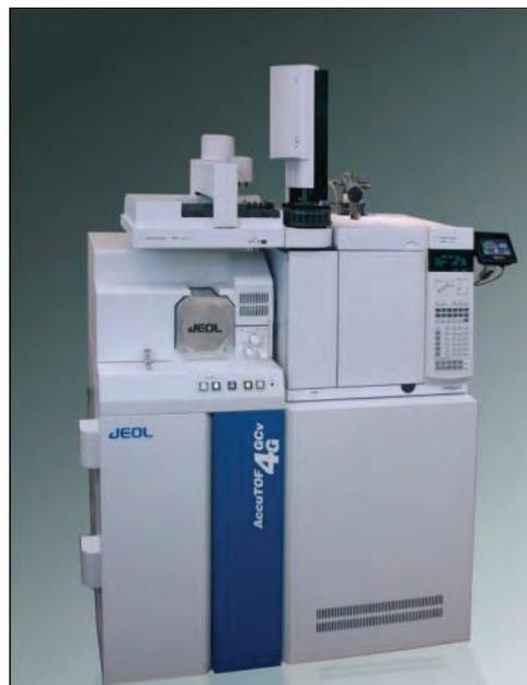
Figure 1. JMS-T100GCV "AccuTOF GCv 4G" GC x GC/HR-TOFMS system
