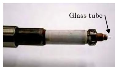
(a) DIP (Direct Insertion Probe)
