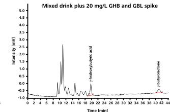
The cocktail was prepared by mixing 80 mL of extra dry Martini with 20 mL of grapefruit juice. After a 1:200 dilution (v/v) with ultrapure water, two aliquots – with and without a 20 mg/L GHB and GBL spike – were subsequently injected.
