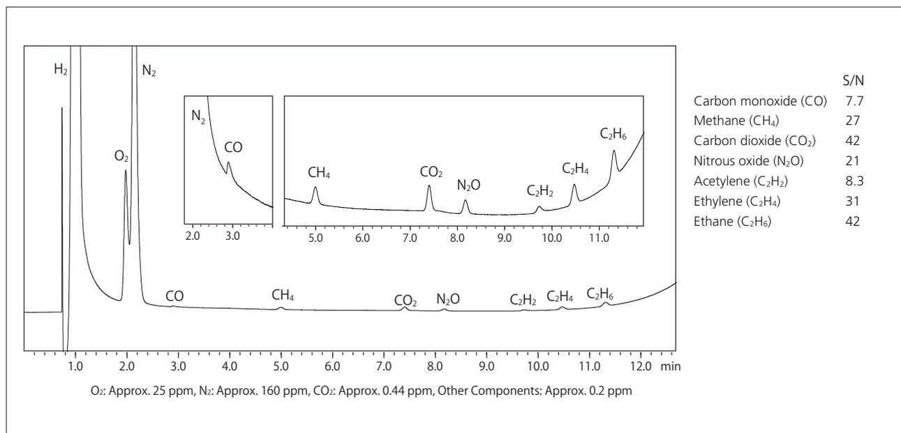
Fig. 2 Chromatogram of Simultaneous Analysis of Impurities in Hydrogen (Micropacked ST Column)
