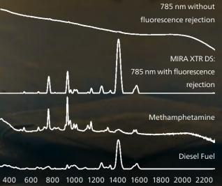
MIRA XTR DS cuts through fluorescence to eXTRact the Raman signal and identify target substances.
