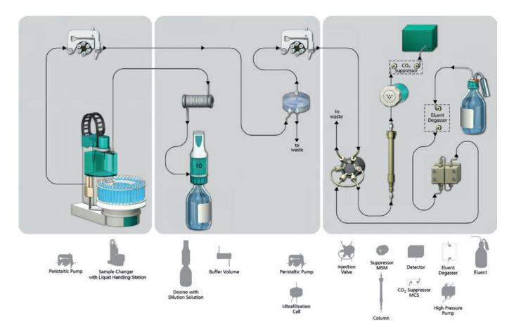
ProfIC Vario 6 Anion: IC system with sequential suppression for anion analysis after Inline Dilution and Inline Ultrafiltration. This system is fully automated and manages the most frequently used sample preparation techniques in routine analysis. It can be calibrated with a single standard.
