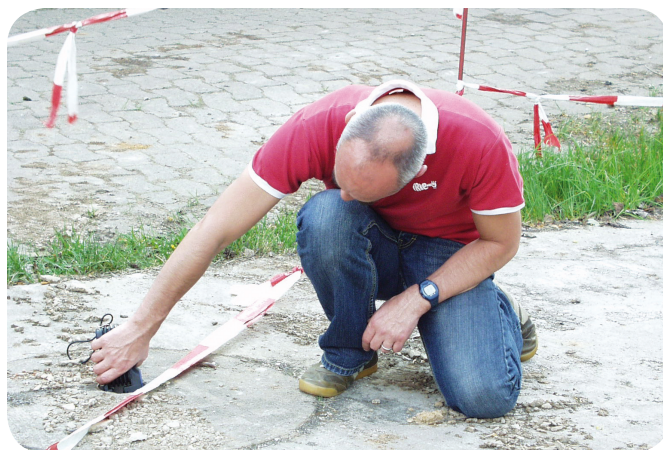
Figure 3: Gas sampling from a dump with hand-held gas detection pump (Dräger ACCURO®)
