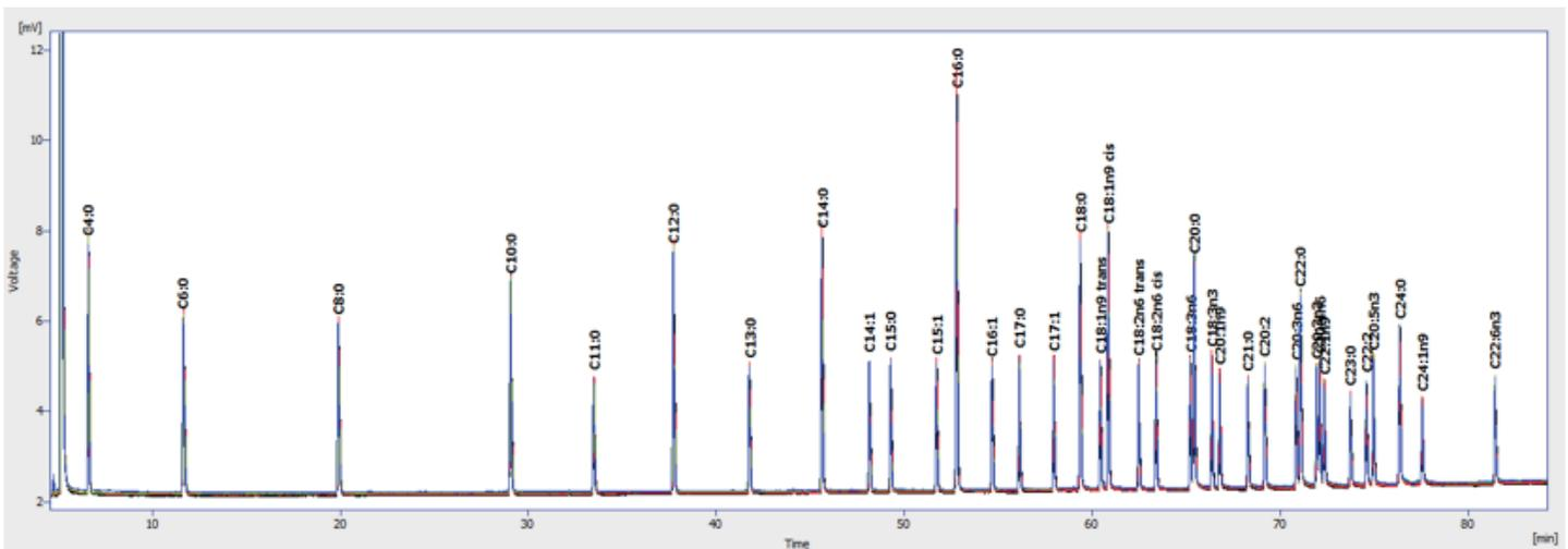
Figure2. Overlay of 6 chromatograms of 37-FAMES MIX
