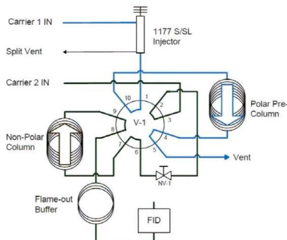
**Fig 1.** Schematic configuration of the analyser during injection
