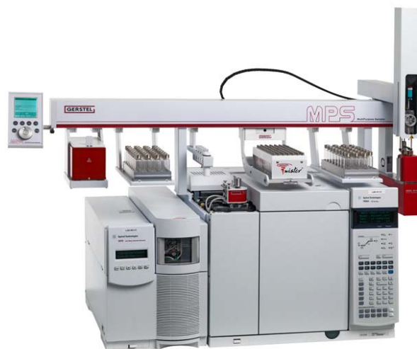
Figure 1. GC/MS system with GERSTEL MultiPurpose Sampler (MPS) used for automation of all sample introduction techniques.
