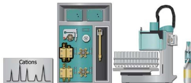
Now assign the following equipment: Define the rack of the connected sample processor, assign the eluent to the IC pump (Pump 2) and define a reasonable start-up time, e.g. 2 minutes. In the analysis link the corresponding pump (Pump 2), (Conductivity Detector 2, Conductivity), injection valve (Injector 2) and column. . Set the temperature of the column oven to 45°C.
