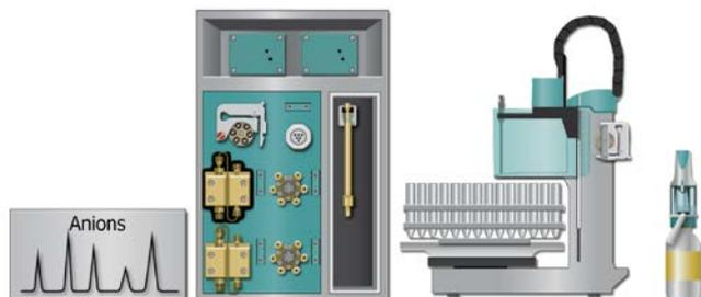
Now assign the following equipment: Assign the suppressor solution to the IC peristaltic pump and set the speed rate to 1, add your Rotor to the MSM and activate the automatic stepping all 10 minutes, define the rack of the connected sample processor, assign the eluent to the anion IC pump (Pump 1) and define reasonable start-up times e.g. 2 minutes. Set the temperature of the column oven to 45°C.
