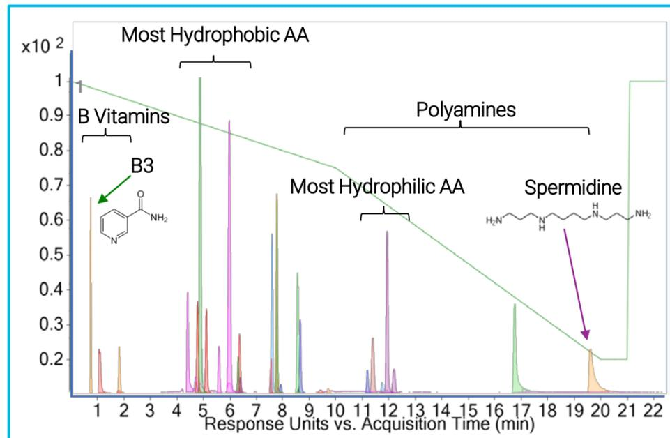
Figure 1. EICs of B vitamin, amino acid, and polyamine standards overlaid with the gradient, illustrating the strength of mobile phase needed to elute various metabolites.
