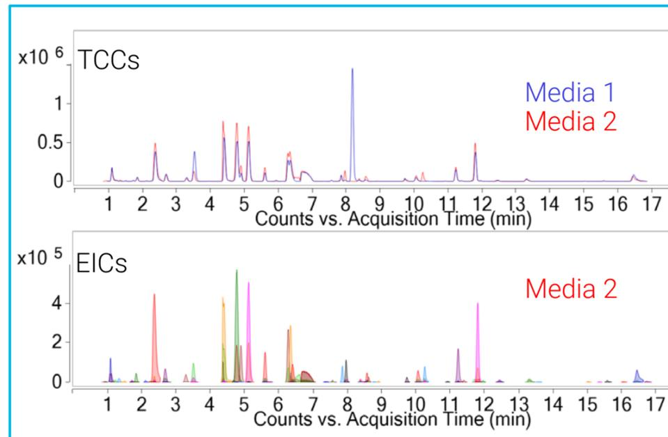
Figure 2. Total compound chromatograms for early timepoint of two media samples (top) and extracted ion chromatograms for all compounds present (bottom).
