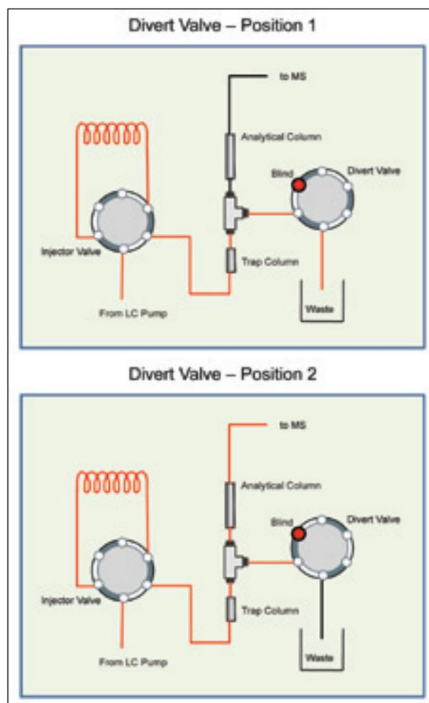
Figure 2. Divert valve positions
