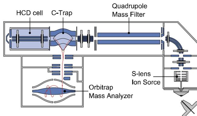
**FIGURE 1. Schematics of the Q Exactive mass spectrometer.**
