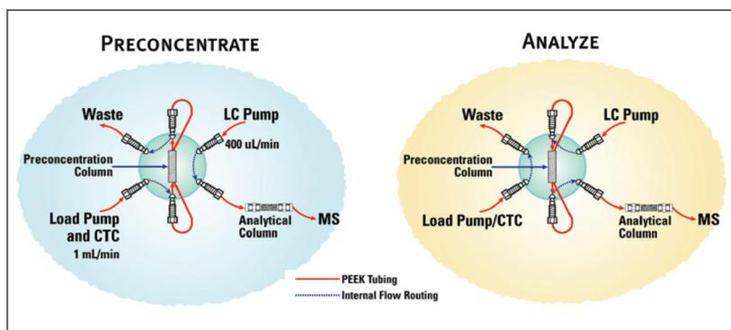
Figure 3. Switching column method for on-line sample injection
