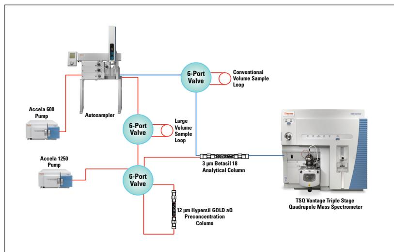
Figure 1. The EQuan pre-concentration LC-MS/MS experimental setup.
