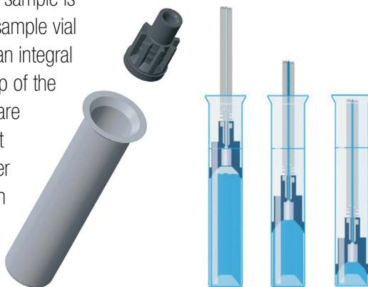
Dionex AS-DV Autosampler sample displacement filtration.
