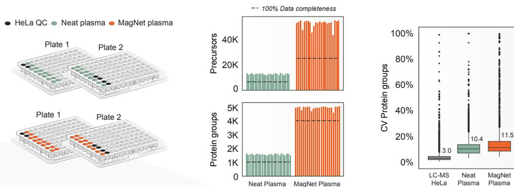
**Figure 3:** Experimental setup and precursor and protein ID levels. CVs representing LC-MS and workflow reproducibility. ~40% of each peptide digest was loaded on Evtips and analyzed with 100 SPD.
