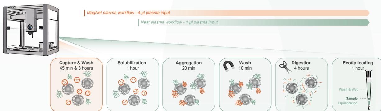
Figure 2: Schematic representation of the OT-2 workflows for neat and MagNet plasma profiling.
