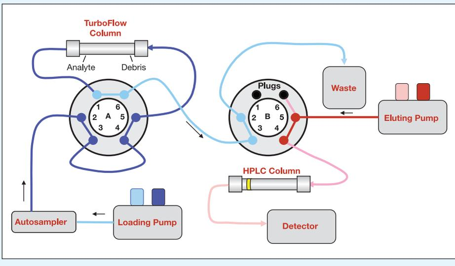
Figure 1: Transcend TLX dual-column configuration
