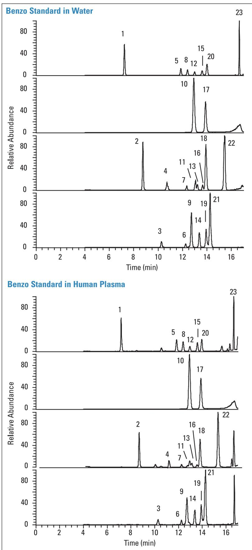
Figure 2: Separation and detection of 23 benzodiazepine standards at 100 ppb concentrations in (a) water and (b) human plasma using the Transcend TLX system coupled to the single quadrupole MSQ Plus mass Detector. Note: This method has 2 min less time for TurboFlow column washing step compared with the stated LC/MS method in Chromatographic conditions.
