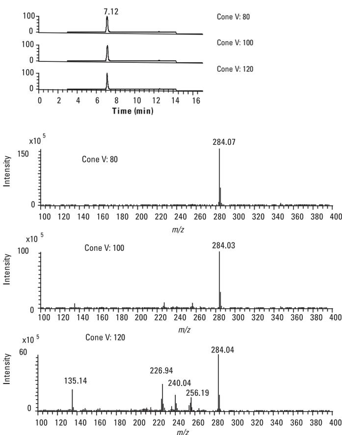
Figure 3: The MS spectra of flunitrazepam and 7-amino-flunitrazepam at 80, 100 and 120 v cone voltage
