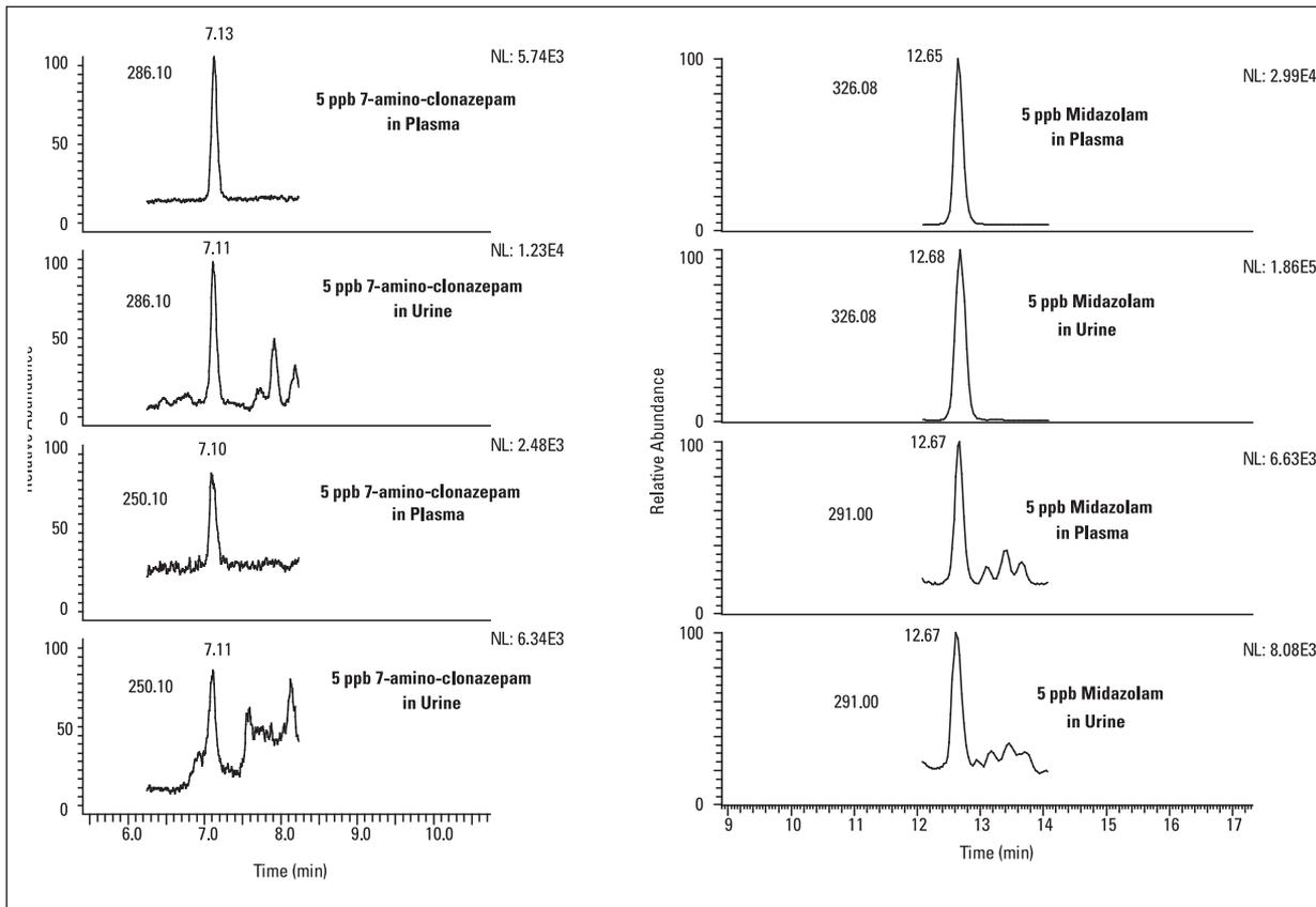
Figure 6: Extracted ion chromatograms of representative benzodiazepines at 5 ppb in human plasma and urine matrices
