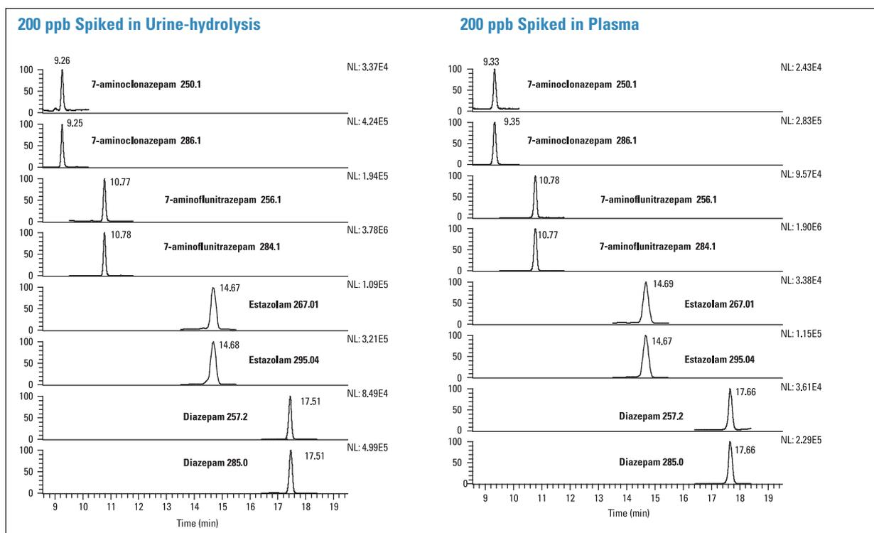
Figure 4. Extracted ion chromatograms of representative benzodiazepines in human plasma and urine matrices. The primary  $m/z$  ion and a confirmation ion were monitored for each benzodiazepine.
