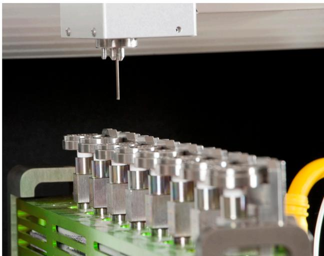
Figure 2: The OSR with controlled atmosphere sampling port technology.
