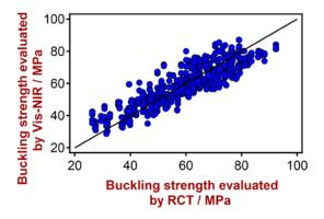
Fig. 6: Correlation plot of reference values from Ring Crush Test (RTC) versus predicted values from Vis-NIR. The buckling strength varies between 26.3 - 92.4 MPa.
