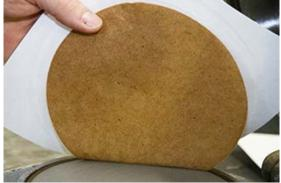
Fig. 1: Standard hand sheets for testing of pulp quality
