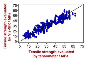
Fig. 7: Correlation plot of reference values from tensometer versus predicted values from Vis-NIR. The tensile strength varies between 8 – 68 MPa.
