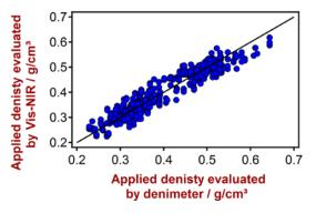
Fig. 8: Correlation plot of reference values from densimeter versus predicted values from Vis-NIR. The applied density values vary between 0.2280 – 0.6437 g / cm<sup>3</sup>.
