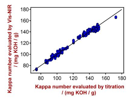
This Application Note shows that visible near-infrared spectroscopy (Vis-NIRS) can simultaneously determine six pulp parameters (kappa number (titration), applied density (densimeter), pulp freeness (CSF), breaking strength (SCT), buckling strength (RCT), and tensile strength (tensometer)) in wood pulp. It is an alternative to conventional lab methods, resulting in a significant reduction in both time to result and chemical waste.
