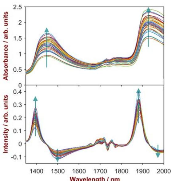
**Fig. 3:** The raw spectra (upper trace) were pre-treated using a Detrend function with a subsequent 1<sup>st</sup> derivative (lower trace). The arrows indicate the trend to higher water concentration.
