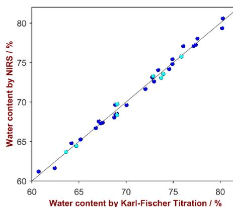
**Fig. 4:** Correlation plot of the moisture concentration determined by Karl-Fischer titration and predicted by NIRS. The blue marks stand for samples used in the calibration set, the turquoise marks are samples used in the validation set.
