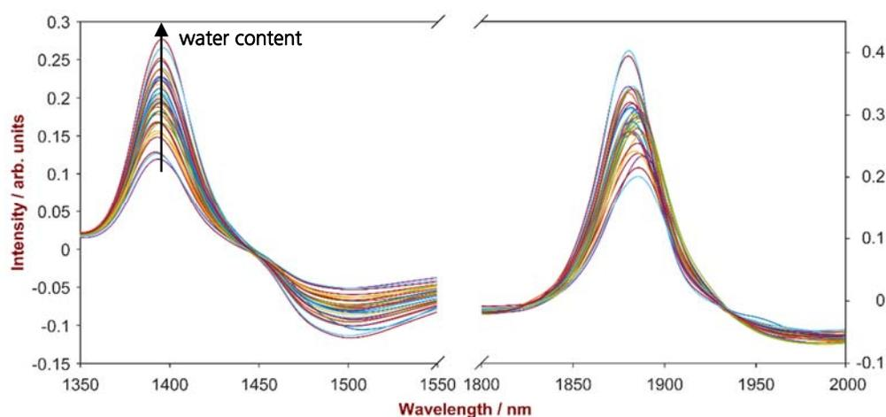
Near-infrared spectroscopy (NIRS) was used as an analysis method for quality control of skin creams. A model for the quantification of the water content was developed based on Karl Fischer titration (KF), enabling fast and reliable at-line analyses and final product quality control.
