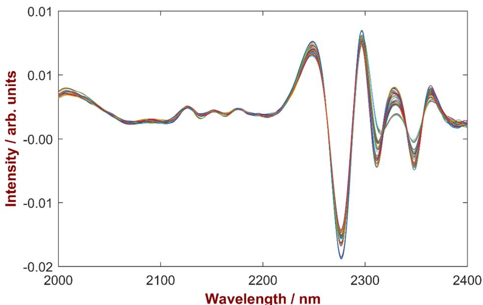
Rapid quality control for toothpaste is achieved by Metrohm's Vis-NIR analyzers. Vis-NIR technology offers significant advantages compared to standard reference analysis. It is a cost effective and safe method because no hazardous chemicals are used.
