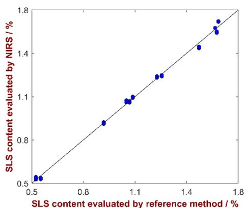
**Fig. 4:** Correlation plot of the SLS content predicted by NIRS versus the reference values. A high correlation is observable.
