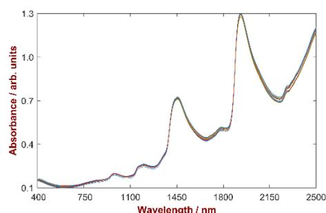
**Fig. 2:** Raw Vis-NIR spectra of 37 toothpaste samples over the full wavelength range.
