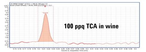
**Figure 5.** HS-SPME GC/Q-TOF analysis of 2,4,6trichloroanisole at 0.1 ng/L. The sensory threshold for TCA is  $\sim 2 \text{ ng/L}$ .
