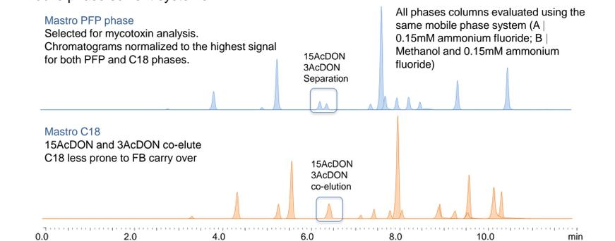
**Figure 3.** 18 Mycotoxins separated on a PFP phase compared to a C18 bonded material using ammonium fluoride as the mobile phase. PFP phases delivered near baseline resolution of 3- and 15 acetyldeoxynivalenol which is not possible on a C18 phase (C18 material can still be used due to preferential ionisation of 3AcDON in negative ion mode).
