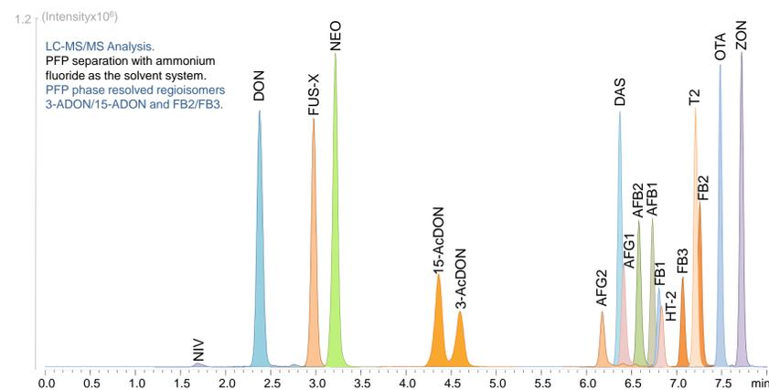
**Figure 1.** MRM chromatograms of 18 mycotoxins using a PFP bonded phase.
