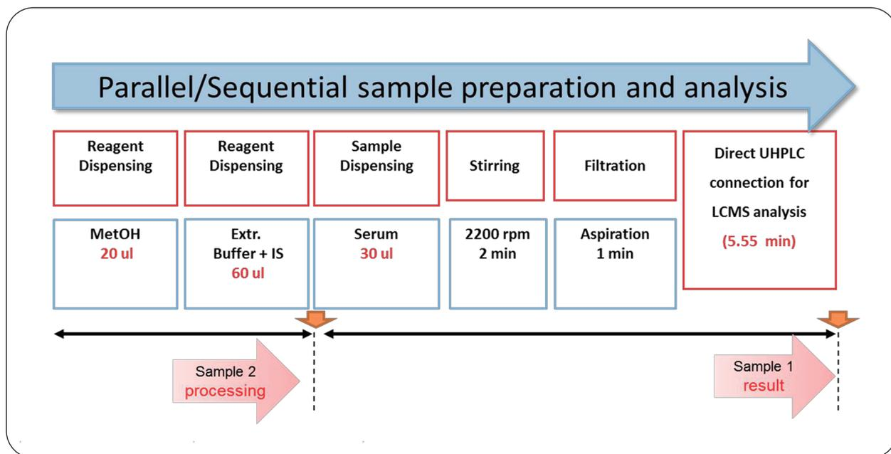
Figure 3: CLAM-2000 fully automated sample preparation and analysis. Due to the overlapped sample preparation the throughput of the instrument was 1 result each 6 minutes for quantification of all Antiepileptics.
