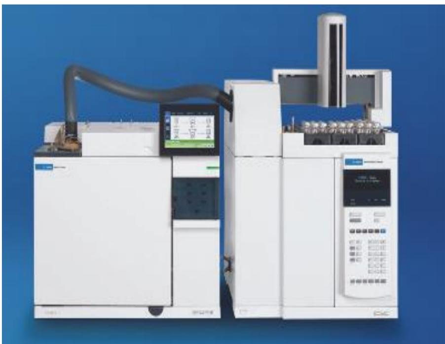
Figure 1: Agilent 7696A Headspace and 8890 Gas Chromatograph
