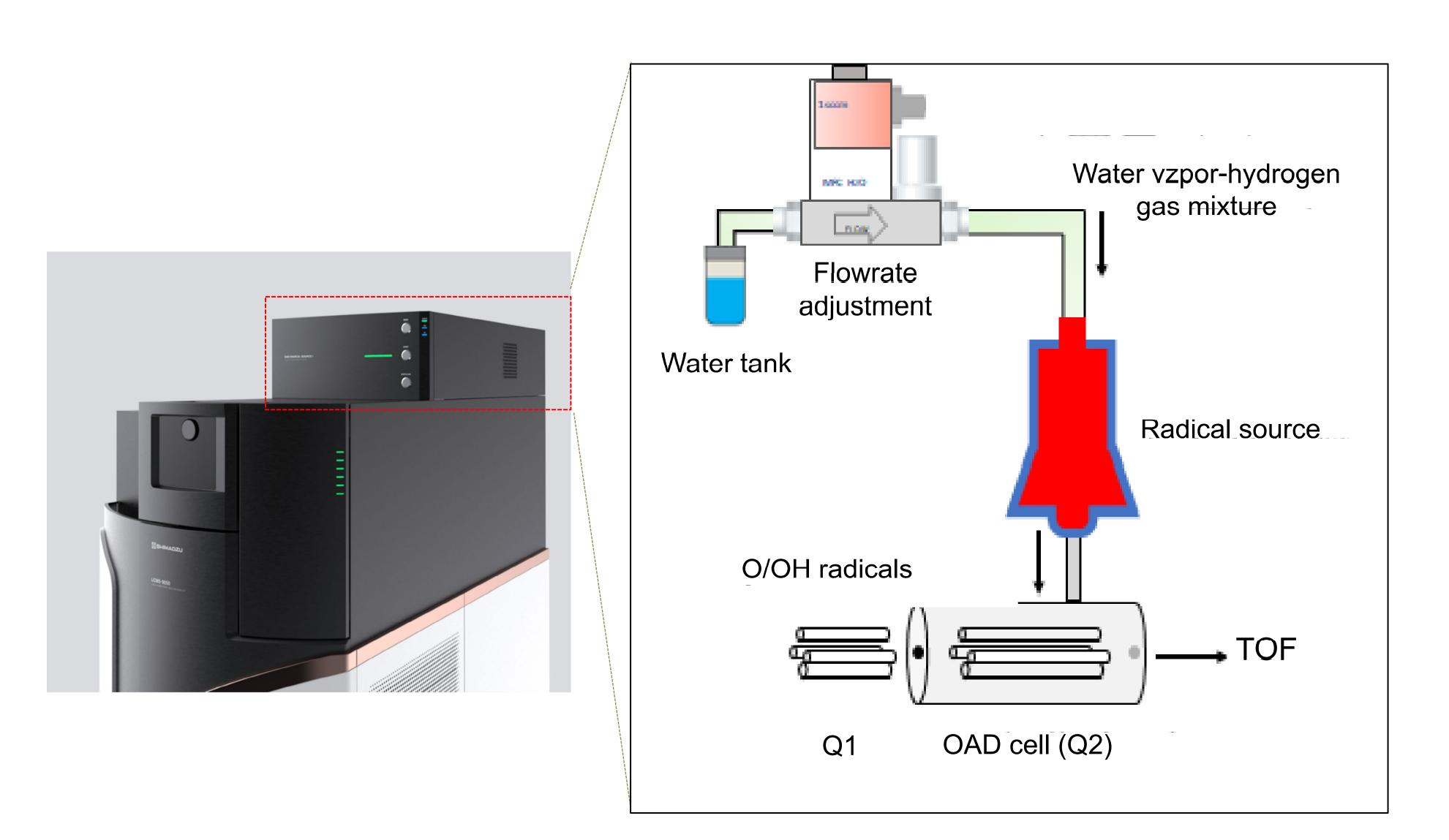
Fig. 1. Shimadzu LCMS<sup>TM</sup>-9050 (Q-TOF) with OAD unit.
