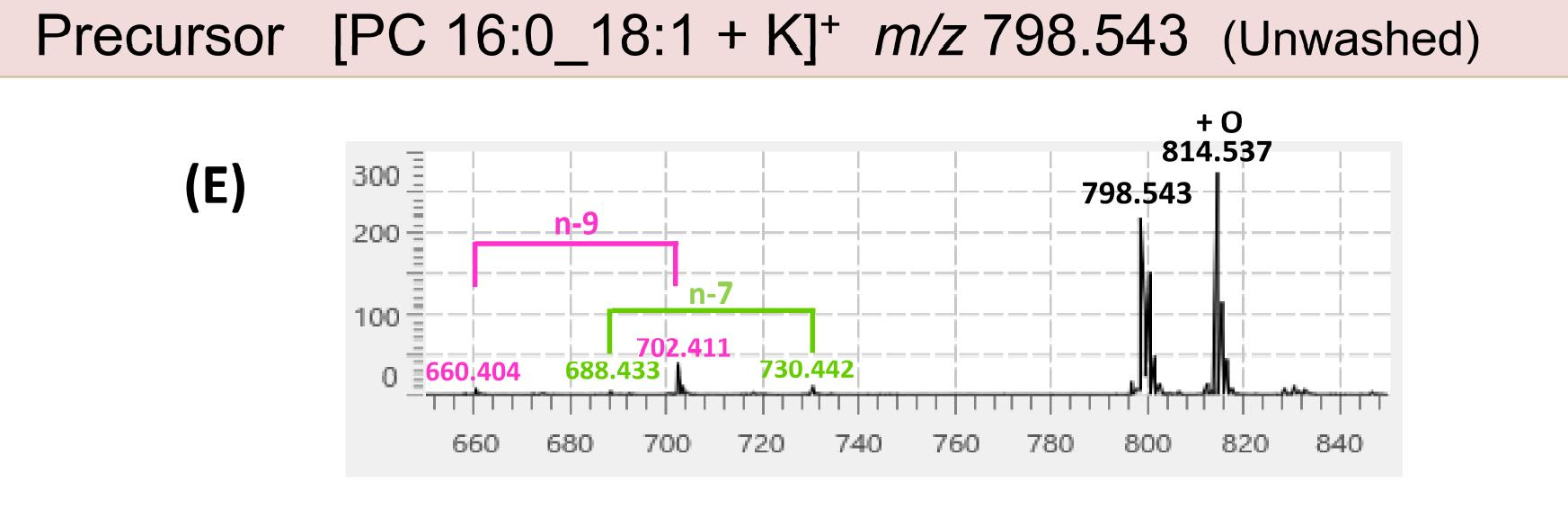
Fig. 4. OAD-MS/MS of PC 16:0\_18:1 in positive ion mode.
