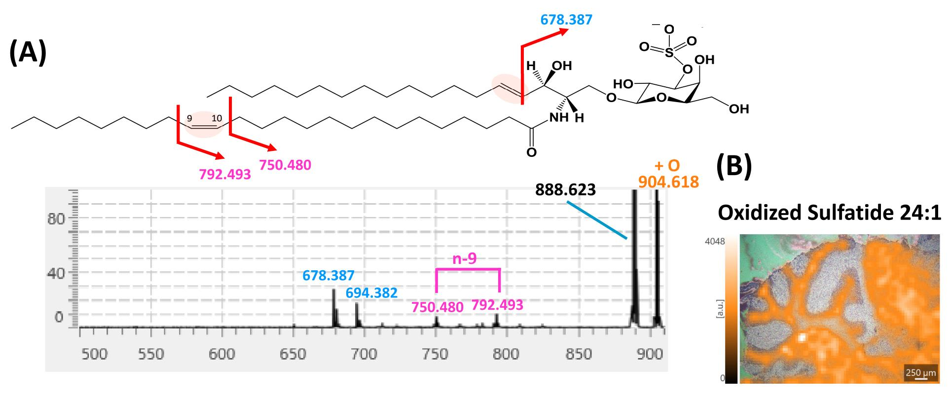
Fig. 5. OAD-MS/MS of Sulfatide 24:1 in negative ion mode.
