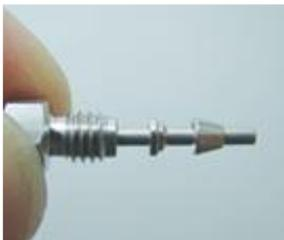
Carefully slide the ferrule components on after the nut. Finger-tighten the assembly while making sure the tubing is completely seated in the bottom of the end fitting.
