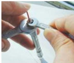
Use a wrench to gently tighten the fitting by 1/4 to 1/2 turn where you want to connect it; this will force the ferrule to seat onto the tubing. Do not over-tighten!
