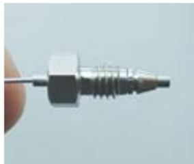
Once you are sure your fitting is complete, loosen the nut and inspect the ferrule for correct position on the tubing.
