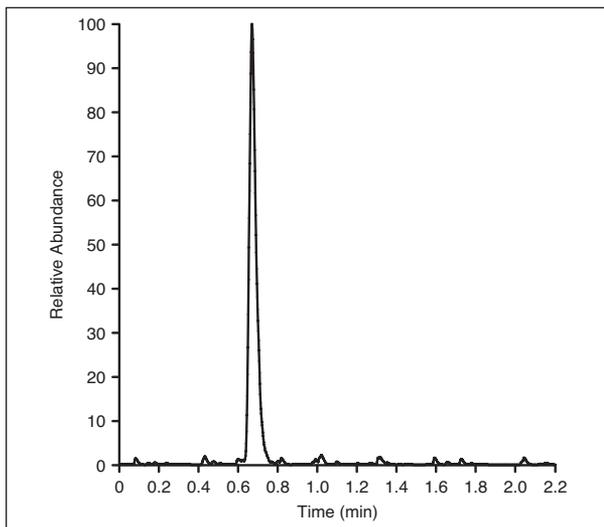
Figure 3. Chromatogram of amlodipine in extracted human plasma.
