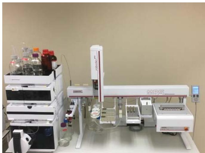
Figure 1. MPS robotic<sup>PRO</sup> Multi-Purpose Sampler with the GERSTEL CF-200 centrifuge option.
