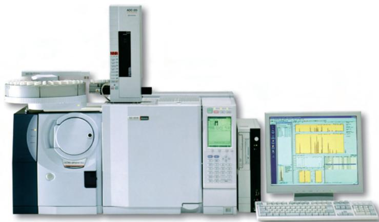
Shimadzu's GCMS-QP2010 Plus
