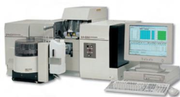
Figure 1: AA-6300 with GFA-EX7i for the electrothermal atomization of Pb, Cd, Pt, Pd and Rh
