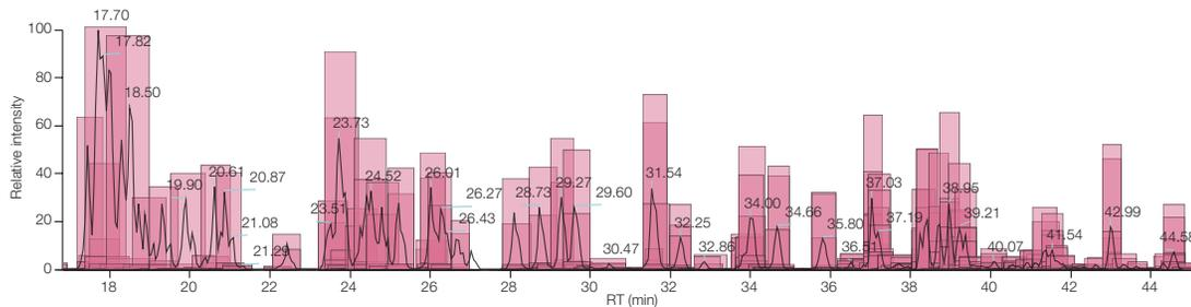
Chromatographic shading is used to quickly and easily identify mRNA digestion fragments throughout the chromatogram. In the above figure identified mRNA digestion fragments are shaded red and pink across the chromatogram for each of the identified mRNA components.
