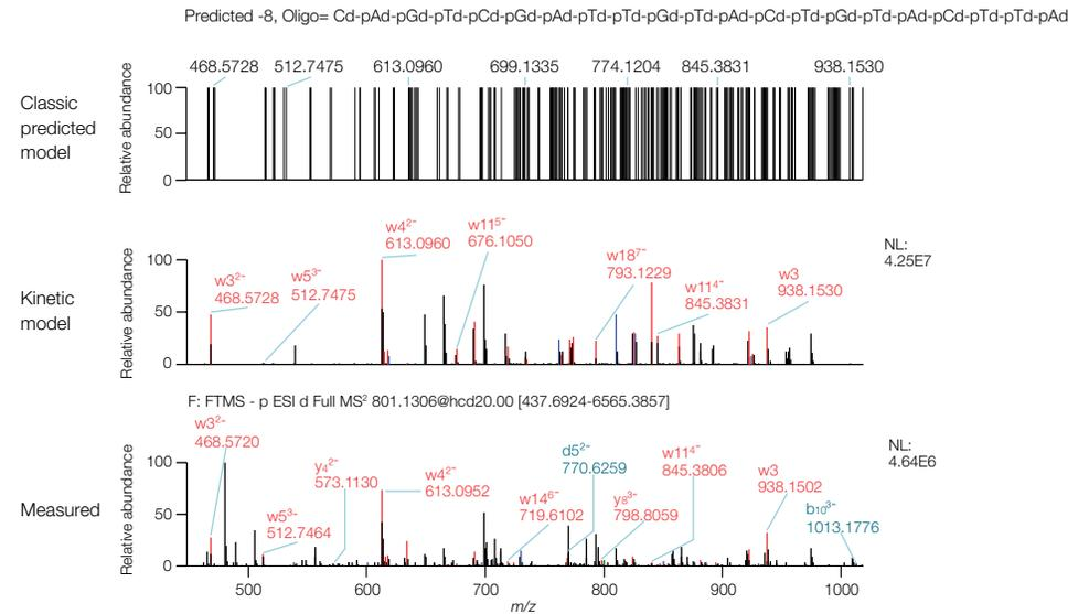
The combination of confident fragmentation prediction and matching MS<sup>2</sup> fragmentation prediction displaying a standard fragmentation *m/z* model (top) and a kinetic model with *m/z* and predicted fragment intensities (middle) versus experimental fragmentation results (bottom).
