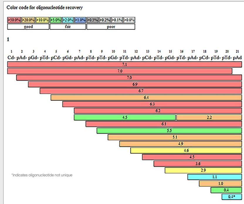
Sequence coverage map display of all identified components within the sample including the full length oligonucleotide product and a wide range of impurities. Chromatographic retention time is displayed for each identified component and each component is color coded based on relative abundance within the sample.
