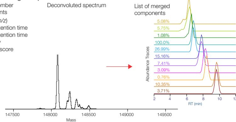
Sliding Window deconvolution provides a key benefit of low abundant variant detection in a single analysis and the ability to accurately detect co-eluting components with different relative abundances. It averages spectra over a succession of sliding windows across retention time, deconvolutes each of these averaged spectra and then merges similar masses to identify components.
