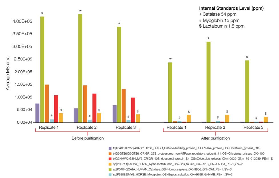
HCPs identified within the sample can be plotted to easily visualize and compare protein quantitation from sample to sample. In the above figure HCPs identified within the sample search in addition to internal standard proteins are plotted before (left) and after (right) sample purification.
