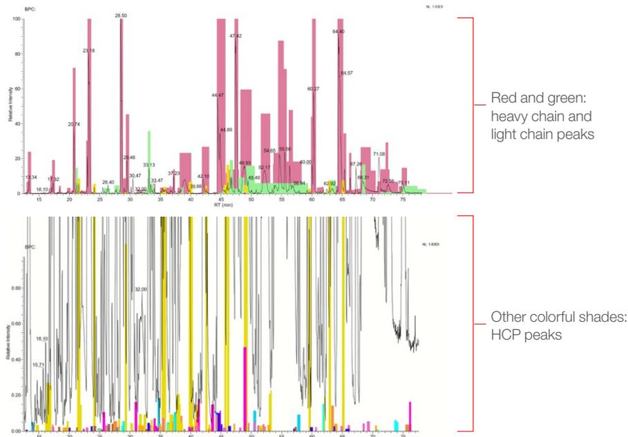
The chromatographic coloring and shading of the components present within a sample provides an easy to use visual tool to simplify chromatographic review. In the above figure components from the light chain (green) and heavy chain (red) regions of the antibody drug product are shaded throughout the chromatogram (top), while HCP components identified within the chromatogram are shaded with a varying range of colors for easy identification (bottom).
