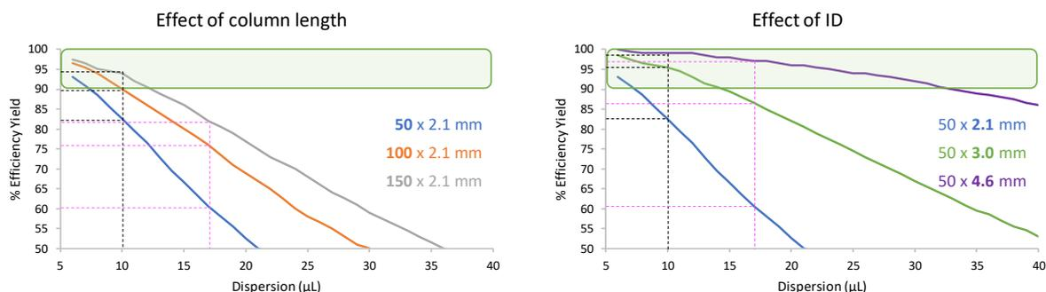
**Figure 2** Theoretical comparison of different column formats packed with 1.7  $\mu\text{m}$  material on the effect of dispersion versus % efficiency yield. The expected efficiency yield for bandwidths of 10 and 17  $\mu\text{L}$  (black and pink trace, respectively) were added to illustrate the necessity for the right instrument for the right column.
