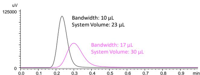
*Figure 1* Operating conditions for system dispersion and example chromatograms of two different systems.
