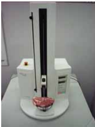
Fig. 8.8.2 Penetrating Strength Test Being Performed on Pork
