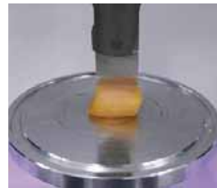
Fig. 8.5.5 Starting Status of Shear Test
