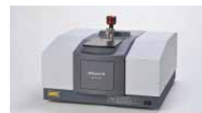
Fig. 7.4.2 Photograph of IRAffinity-1 with MIRacle 10 ATR Accessory Attached
