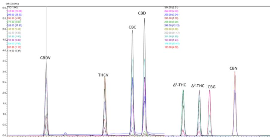
**Analysis of 11 Cannabinoids with Shimadzu's GCMS**
