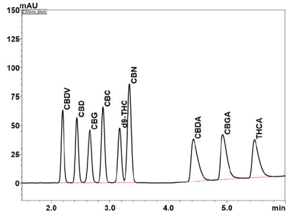
**Analysis of 9 cannabinoids with Shimadzu's Nexera UC SFC system**
