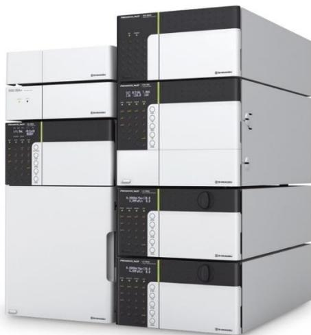
The ion chromatograph described in EPA Methods 300.0 and 300.1 consists of an autosampler, a pump, an injection valve, a column and guard column, a suppressor, and a conductivity detector. Separation of analytes takes place on the column while the guard column helps to prevent contamination of the column.
