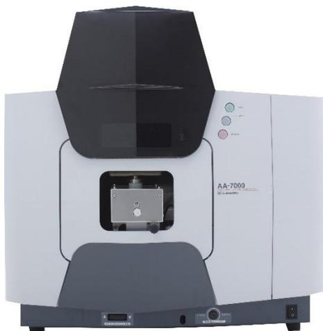
[Atomic Absorption Spectrophotometry \(AAS\)](#) is a single-element technique used to measure metals in aqueous samples. AA is the instrument of choice for laboratories running fewer than six elements per sample in only a few samples per day because of its great flexibility and lower operating costs.
