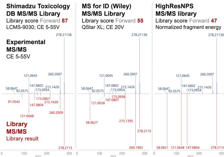
**Figure 1.** Library results for venlafaxine (antidepressant; C<sub>17</sub>H<sub>27</sub>NO<sub>2</sub>, precursor m/z 278.2115) using multiple data repositories to help increase reporting confidence in compound identification. Although the data repositories use different QTOF platforms and different fragment ion intensities (CE spread 5-55V, fixed CE 20V and normalized fragment ion intensity) each MS/MS library can provide positive evidence for compound identification.
