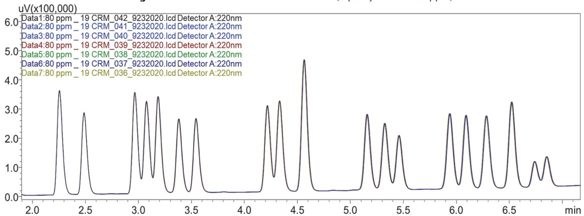
**Figure 3:** 19-cannabinoid mixture repeatability and overlay of seven injections (5 µL injection at 80 ppm)
