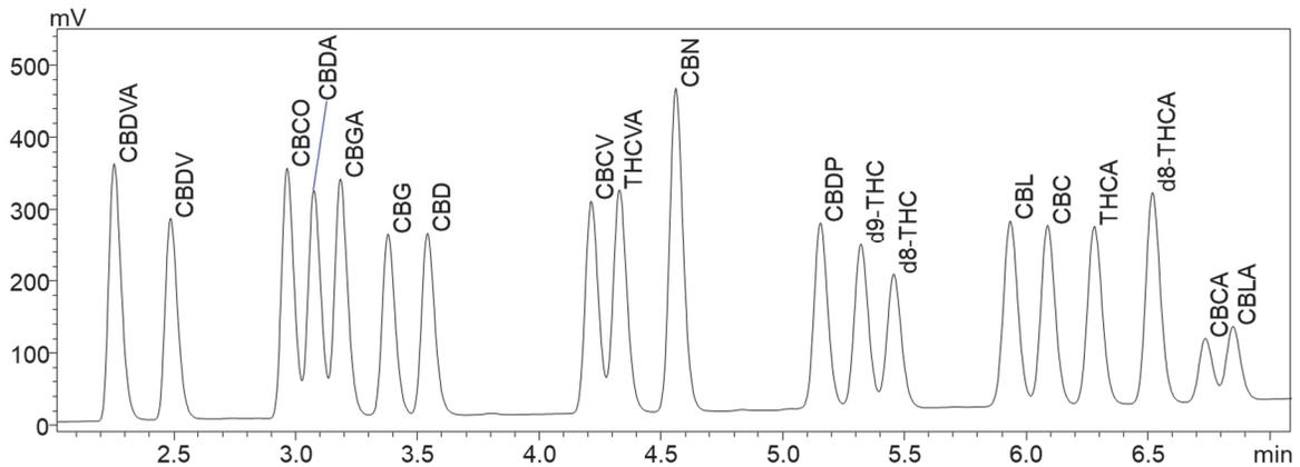
**Figure 2:** 19-cannabinoid mixture resolution (5 µL injection at 80 ppm)
