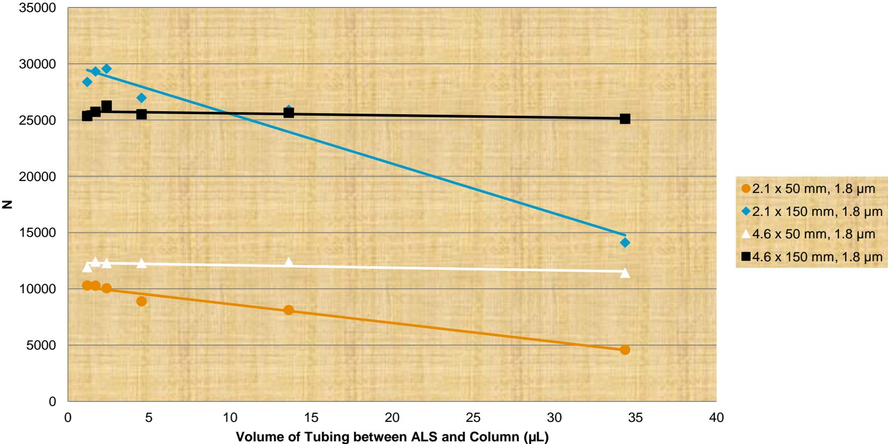
The above scatter plots compare the effects of column length and internal diameter on the ECV impact on efficiency; length has a lesser effect, while the column's internal diameter's effect is much greater
