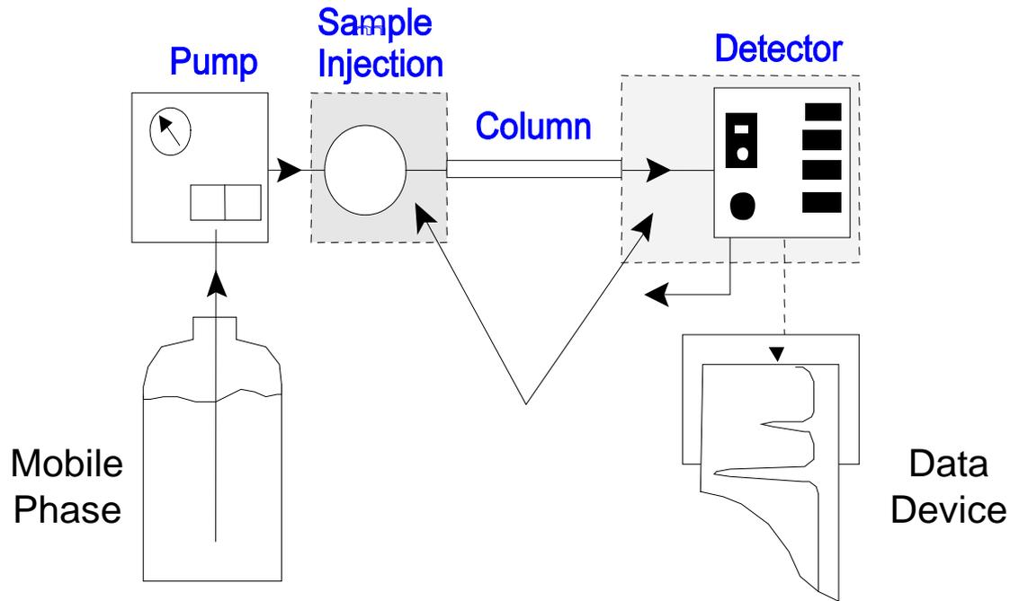
The instrument schematic above depicts where extra-column volume can occur, thus effecting instrument and column performance.
