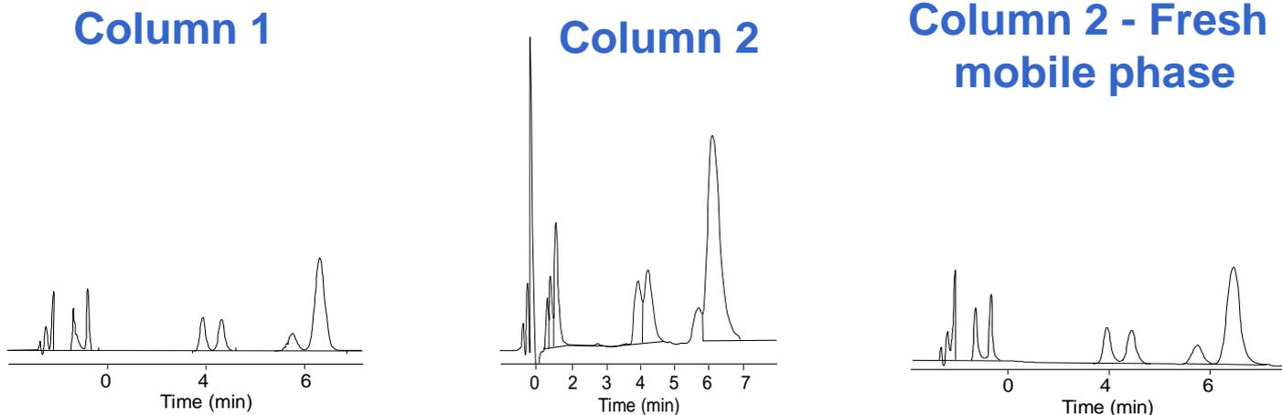
*“I have experimented with our mobile phase, opening new bottles of all mobile phase components. When I use all fresh ingredients, the problem ceases to exist, and I have narrowed the problem to either a bad bottle of TEA or phosphoric acid. Our problem has been solved.”*
