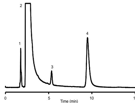
**Column washing eliminates the peak splitting, which resulted from a contaminant on the column.**
