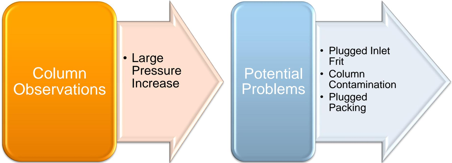
Note: Low pressure is typically a connection or LC issue; unless the column has been improperly used and disassembled or lost all its packing.
