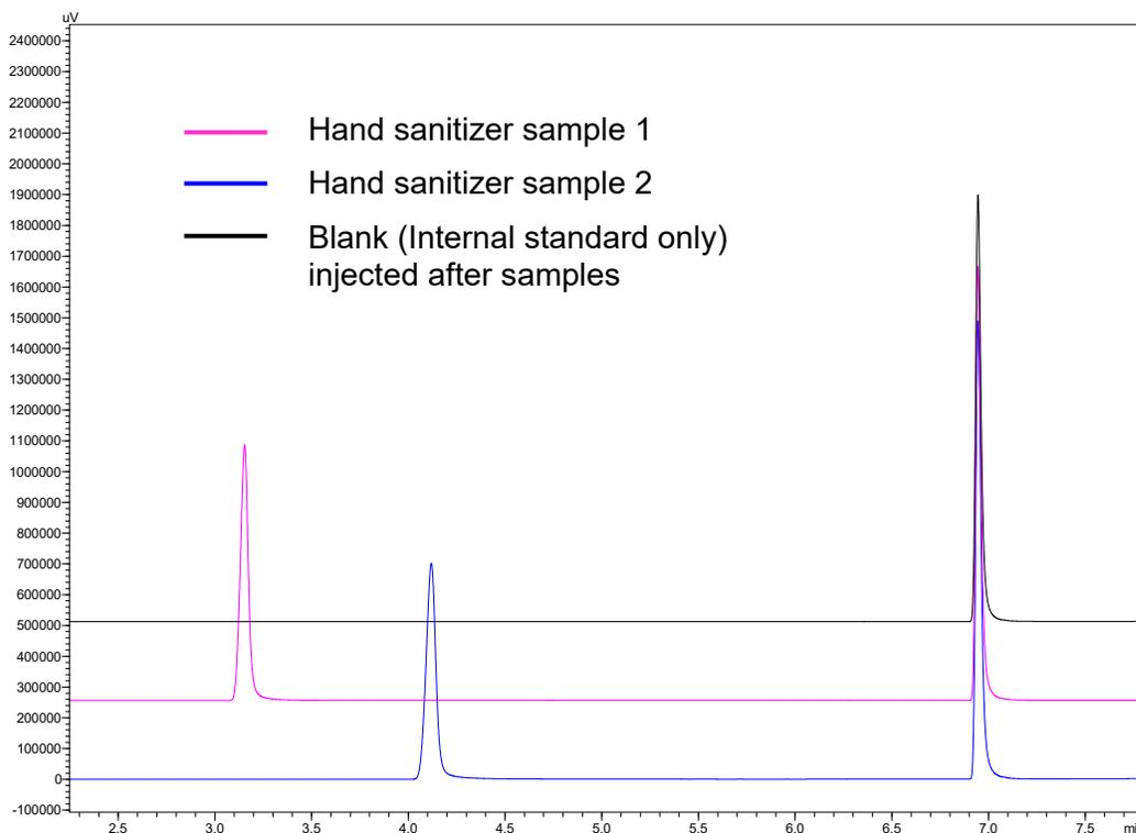
**Figure 3:** Chromatograms of hand sanitizer samples and a blank injected after the samples. No carryover of analytes was observed
