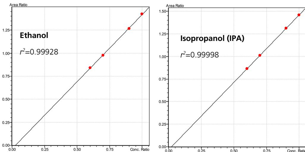
Figure 2: Four-point calibration curves for ethanol and IPA
