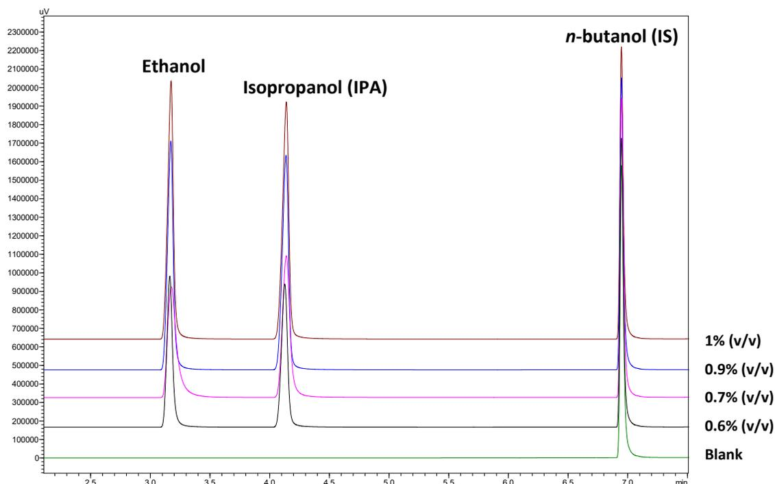
Figure 1: Chromatograms of calibration standards and water blank with IS (*n*-butanol)
