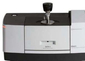
**Fig. 1: IRspirit™ FTIR with QATR™-S**
