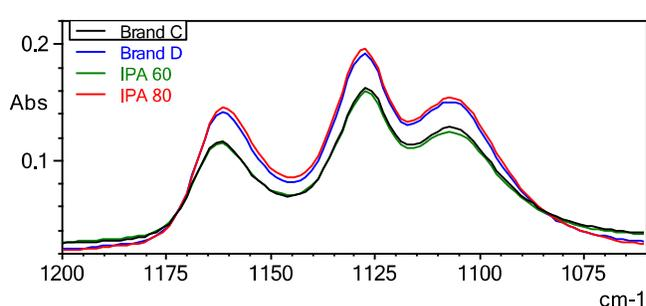
Fig. 4: IR Spectra of Brand A and B with 60% and 80% Ethanol Standards (left) and Brand C and D with 60% and 80% IPA Standards (right)
