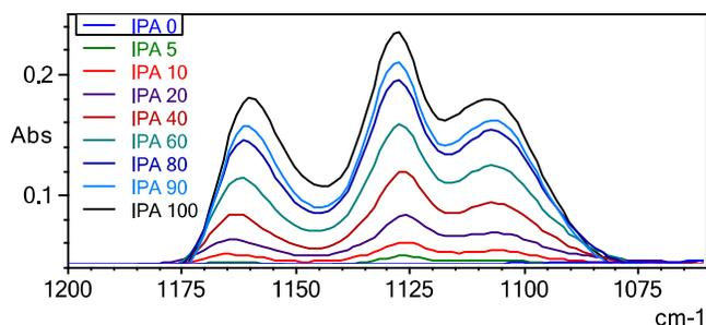
Fig. 3: IR Spectra of Ethanol Standards (left) and IPA Standards (right)
