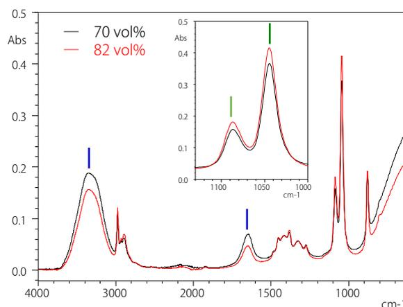
Fig. 3 IR Spectra of Ethanol Standards (70, 82 vol%)
