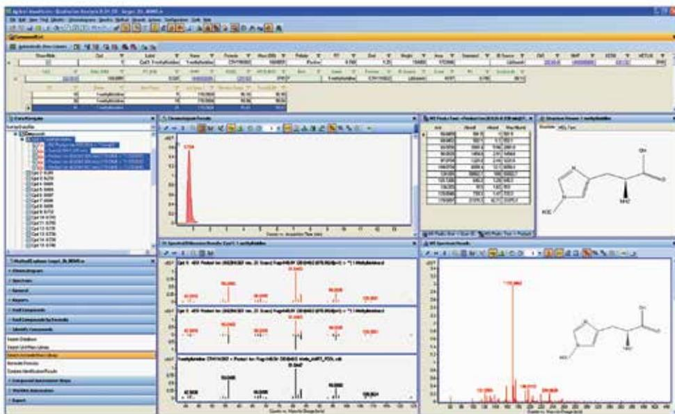
**Figure 74.** MassHunter Qualitative Analysis, a component of the popular MassHunter Workstation software suite, uses accurate-mass, retention-time, isotope-pattern, and MS/MS data to generate the highest-confidence, metabolite identifications
