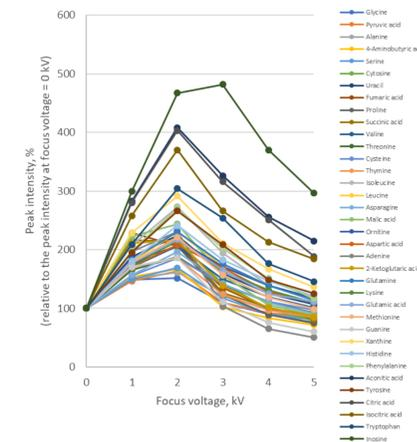
Figure 3 The relationship between focus voltage and peak intensity
