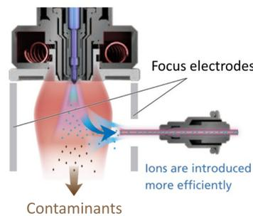
Figure1 The concept of the IonFocus Unit
