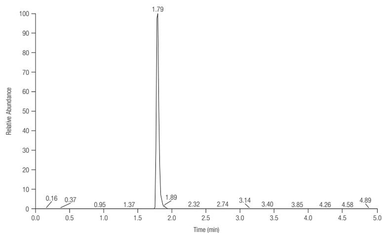
Figure 7. 100 ng/mL standard of corticosteroid d8 (internal standard).
