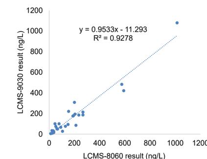
Figure 2. Comparison of quantitative results across two LC-MS/MS platforms: triple quadrupole (LCMS-8060) and Q-TOF (LCMS-9030) showed good correspondence.
