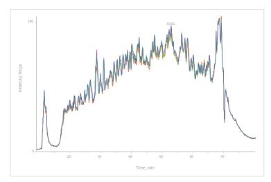
The Total Ion Chromatograms (TICs) of 10 replicate injections of depleted plasma analyzed by MS/MS<sup>ALL</sup> with SWATH Acquisition overlay with excellent reproducibility for highest quantitative robustness.
