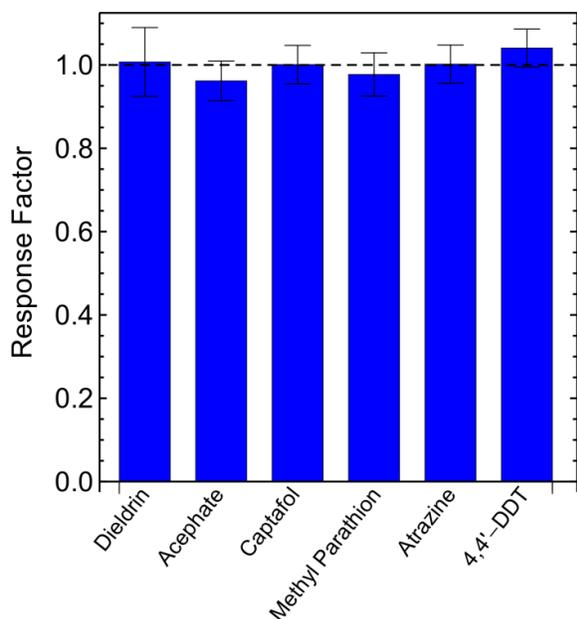
**Figure 4.** Response factors obtained for six pesticides analyzed with the Polyarc™ reactor
