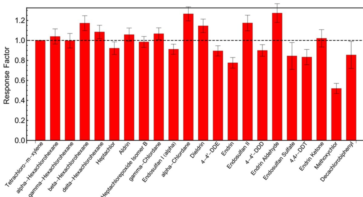
**Figure 5.** Response factors obtained for a 22-component organochlorine pesticide mixture (200 µg/mL in hexane:toluene 1:1) with a poor absolute injection of analytes onto the column.
