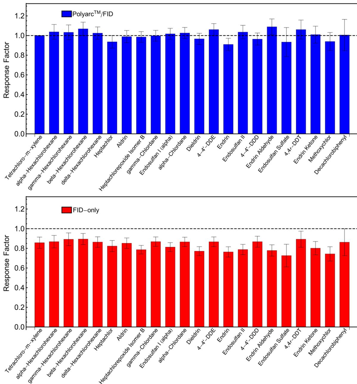
**Figure 3.** Response factors obtained for a 22-component organochlorine pesticide mixture (200 µg/mL in hexane:toluene 1:1) using the Polyarc™ reactor (top) and FID-only (bottom).
