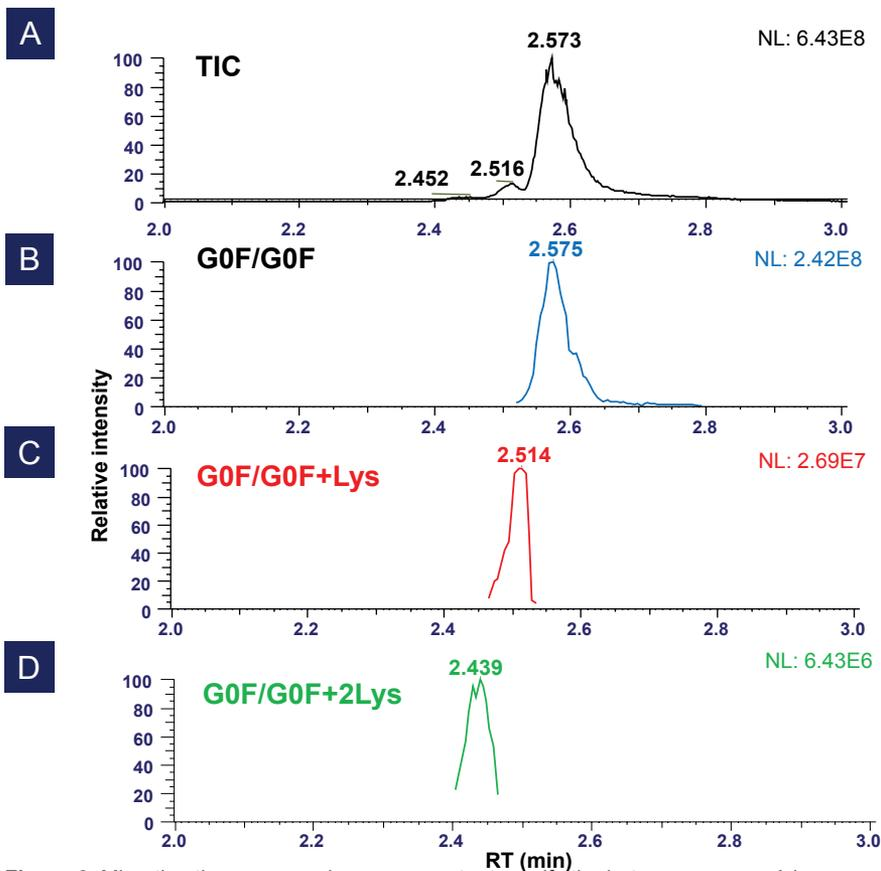
**Figure 6.** Migration time was used as a parameter to verify the heterogeneous mAb in an example of specific glycosylation form G0F/G0F. A) Total Ion Chromatogram (TIC) in a 4 min run of NIST mAb. B) TIC from the specific form of G0F/G0F. C) TIC from the specific form of G0F/G0F+Lys. D) TIC from the specific form of G0F/G0F+2Lys
