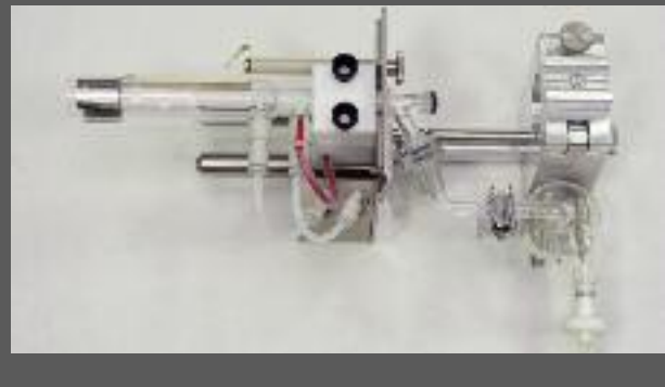
FIGURE 2. Modified ELEMENT 2/XR torchbox for GC analysis.
