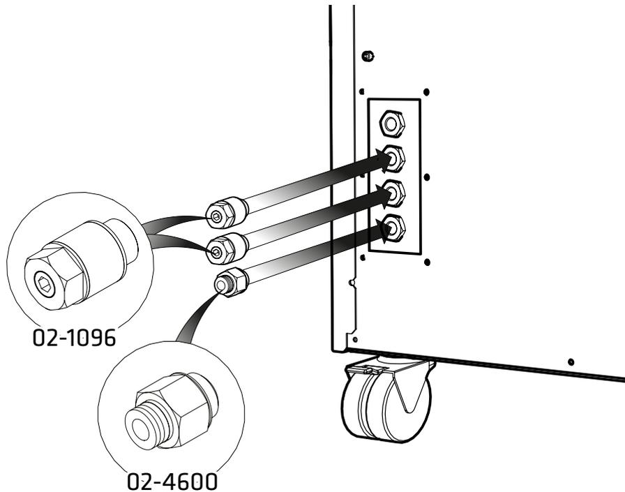
**Select the 6mm Push Fit Fitting 02-4600** and attach to the **Drain port** at the rear of the generator. **Attach the Flow Control Silencer 02-1096** to the **Nitrogen and Air ports**.
