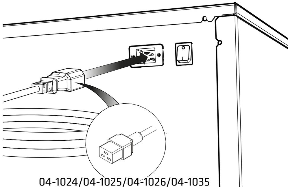
Select the appropriate power cable from the fittings kit and **plug the IEC 60320/C19 cable into the power input** at the rear of the generator.
