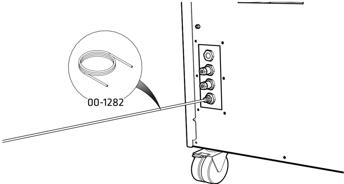
Connect the **6mm Polyethylene Tubing 00-1282** to the **6mm Push Fit Fitting 02-4600**. Fit the other end of the tubing to a suitable drain connection or container. The container **MUST NOT** have an airtight seal as water and air will be expelled periodically under a slight pressure.
