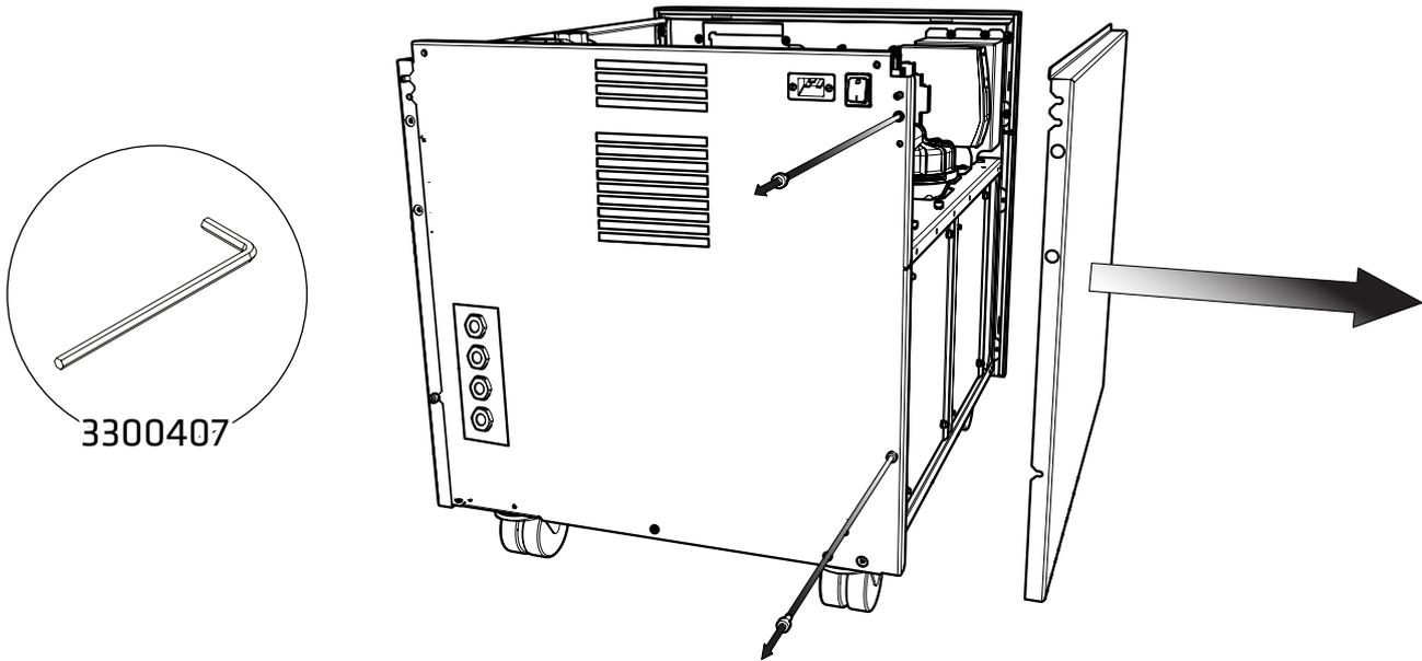
Once the top plate has been removed, use the **4mm Hex Key 3300407** to loosen the **two cap screws** fixing the right-hand side panel to the rear of the generator, then **tilt outwards and slide backwards to release the side plate from the generator.**
