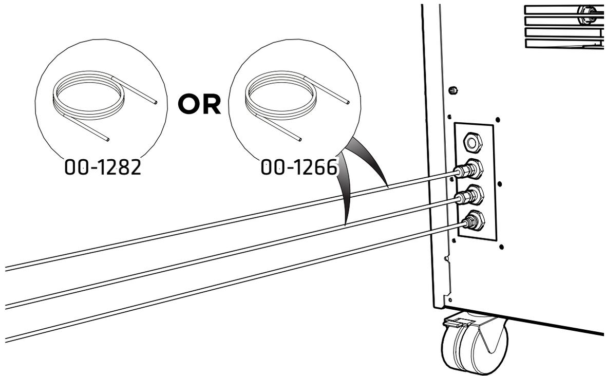
Attach the appropriate sized **tubing** to the fitting attached to the **Nitrogen and Air ports** and connect the other end to the **gas inlet of your instrument**.
