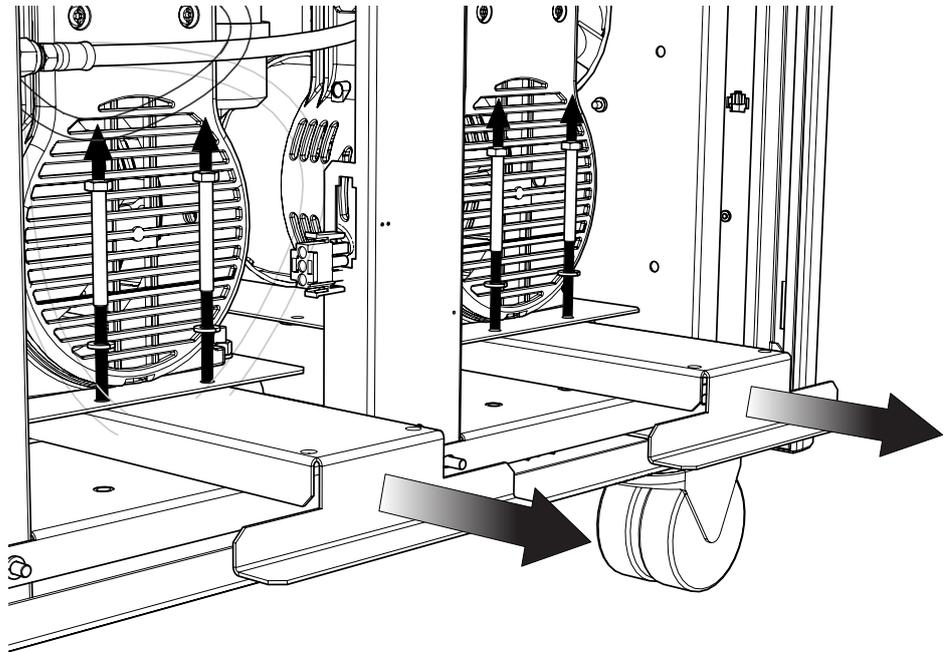
The transit brackets are located below the compressors and have stickers on them stating 'Remove before use'. To **remove the transit brackets**, use a **10mm spanner** to **remove the two screws on each bracket** as indicated, then **slide the brackets out** from underneath the compressors. **There are three brackets in total. Please retain the brackets and screws for future transportation.**
