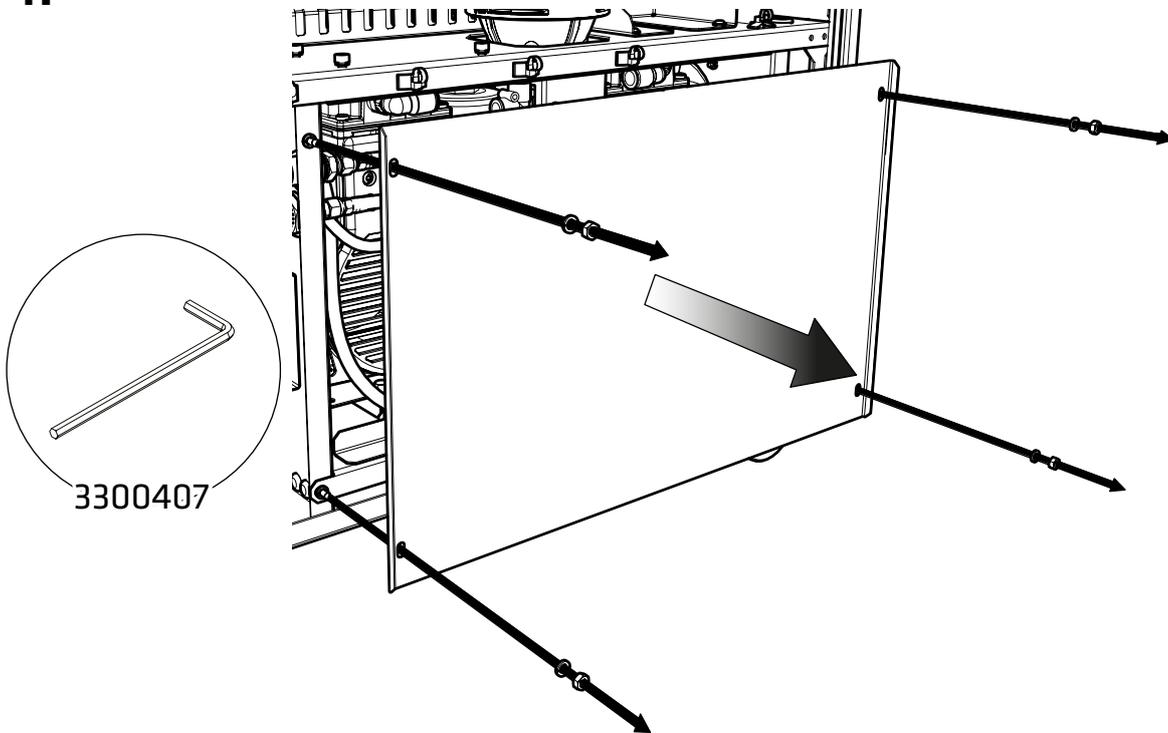
With the right-hand side plate removed, use the **4mm Hex Key 3300407** to **remove the hex bolts** holding the compressor door in place, taking care to **retain the spring washers.**
