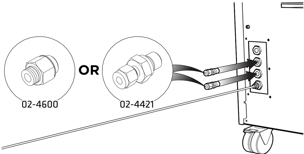
Depending on the size of the inlet on the instrument, select either the 1/4" **Compression Fitting 02-4421** or the remaining 1/4"- 6mm **Push Fit Fittings 02-4600** and connect these to the **Nitrogen and Air ports**.
