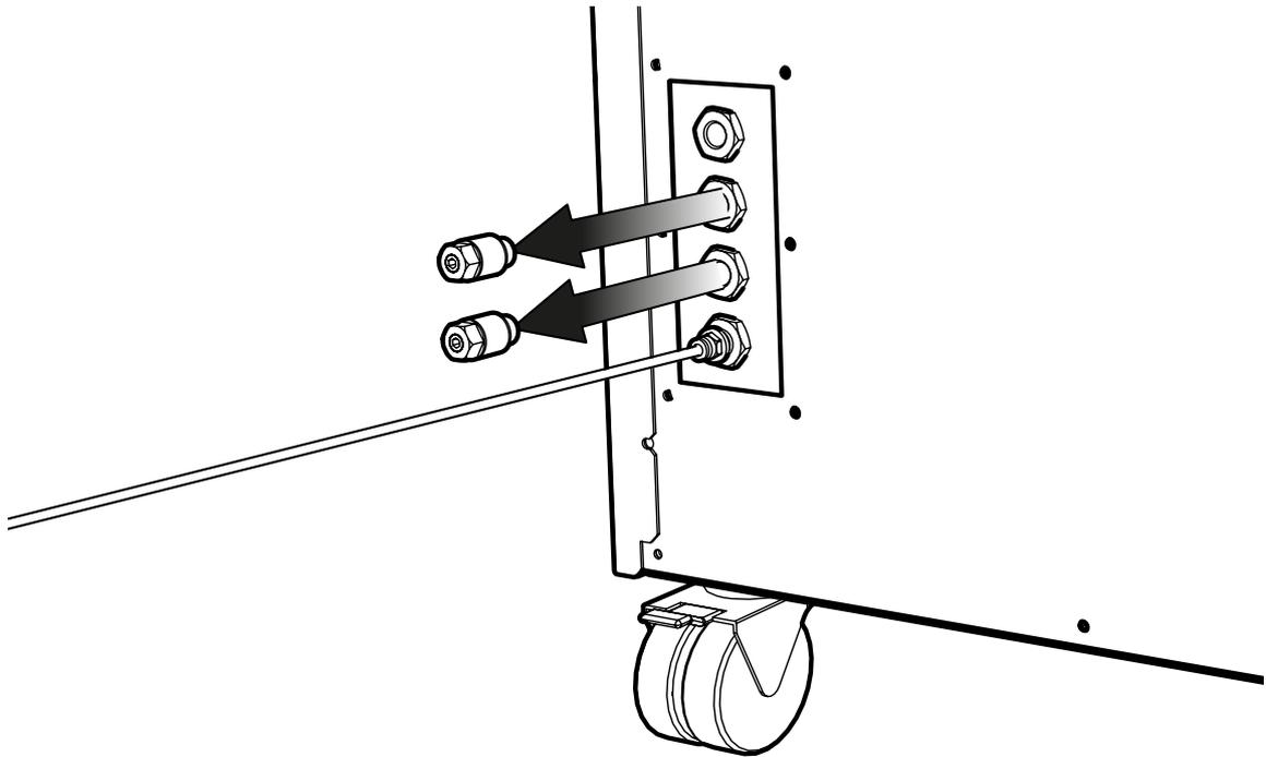
Once the pressure has dissipated the **silencer fittings** can be removed from the **Nitrogen and Air ports**.
