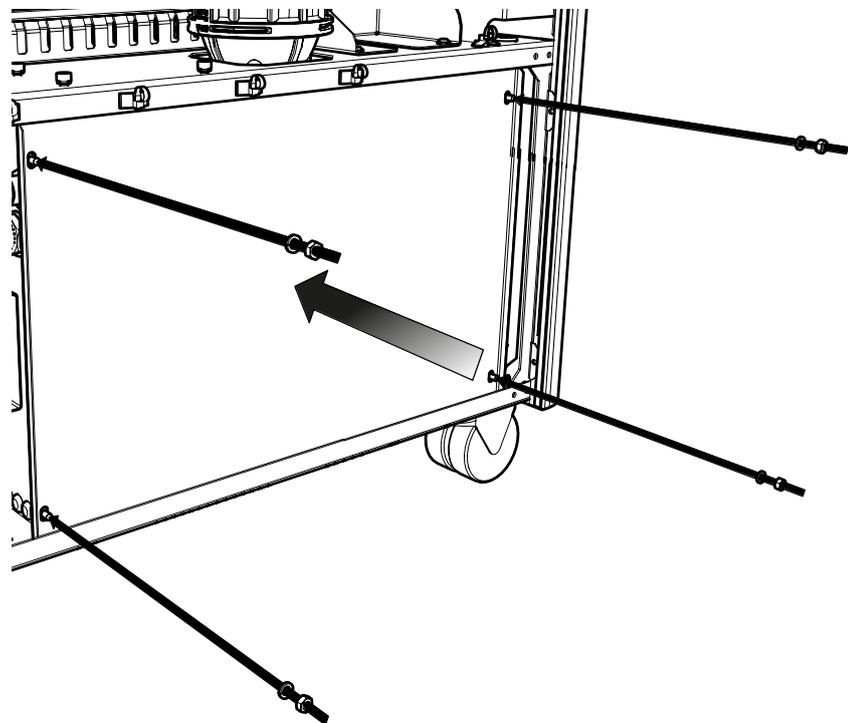
**Replace the compressor doors**, again using the **4mm Hex Key 3300407**.
