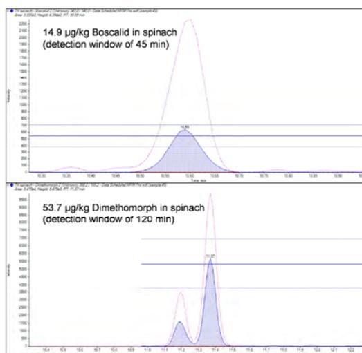
**Figure 7.** Examples of using the Flexible Window Width in a Scheduled MRM Pro Algorithm: the window for Boscalid was set to 45 sec and Dimethomorph was detected using a wider window to detect both isomers together
