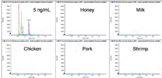
Figure 6. Blank matrices tested for tetracyclines (10 µL injection)
