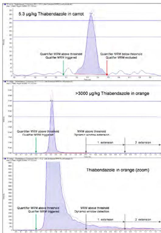
**Figure 8.** Examples of MRM-triggered MRM and Dynamic Window Extension: the qualifier MRM transition is automatically triggered when the qualifier MRM transitions exceeds the threshold set in the *Scheduled MRM Pro* Algorithm, the detection window is automatically extended if the MRM signal is above the threshold at the end of the detection window
