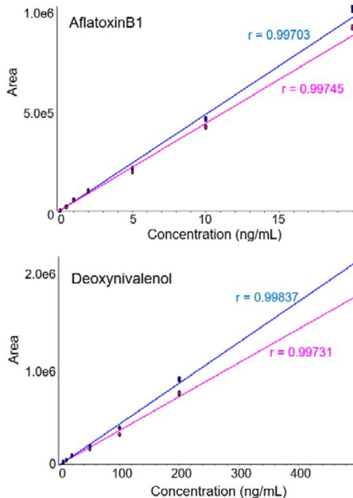
**Figure 4. Calibration Curves for AflatoxinB1 and Deoxynivalenol.** Calibration curves were generated from 5 to 500 ng/mL. Two MRM transitions were monitored: fragment 1 (blue) and fragment 2 (pink). R-values shown for both transitions for both representative analytes are >0.99, demonstrating excellent linear range and response for the assay
