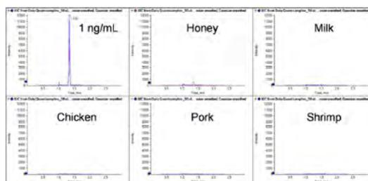
Figure 5. Blank matrices tested for Chloramphenicol (50  $\mu\text{L}$  injection), the honey sample had a trace contamination with Chloramphenicol below the LOQ of 0.05 ng/mL (0.25  $\mu\text{g}/\text{kg}$  in matrix after 5x dilution)
