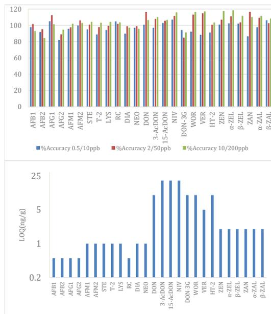
**Figure 1. Accuracy and LOQ Values Shown for the Panel of Mycotoxins.** Limits of Quantitation (LOQ) of all mycotoxins were found between 0.5 ng/g and 20ng/g. Accuracy assessed over three concentrations ranged from 80% to 120%. These measurements of performance demonstrate excellent sensitivity and accuracy for this assay
