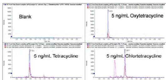
Figure 2. Sensitivity of a 5 ng/mL standard of tetracyclines (injection volume of 10  $\mu\text{L}$ )
