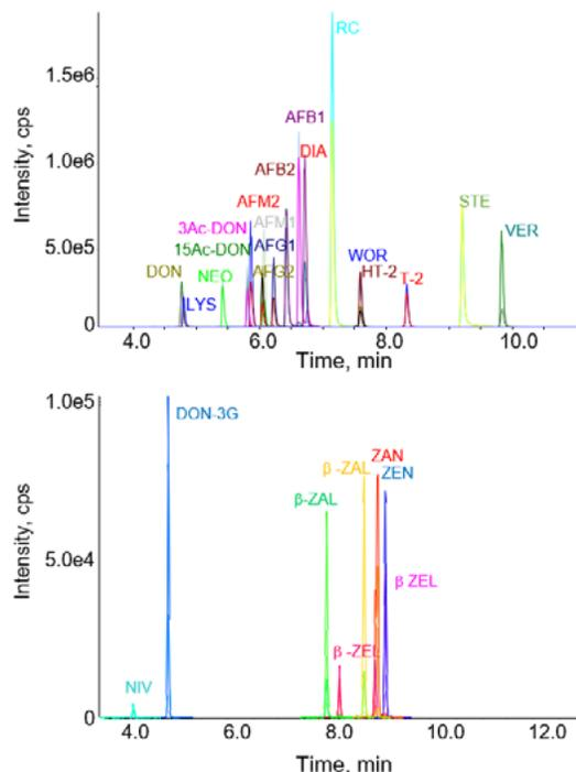
**Figure 2. Chromatographic Profile for 26 Mycotoxins.** Both positive and negative modes were analyzed simultaneously during a single sample injection, allowing all 26 mycotoxins to be analyzed in one data acquisition method. (Top) 18 mycotoxins were collected in ESI positive mode (top) and 8 mycotoxins were collected in ESI negative mode (bottom)
