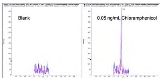
Figure 3. LOQ for Chloramphenicol of less than 0.05 ng/mL with an injection volume of 50  $\mu\text{L}$ , allowing 10x dilution of matrix extracts
